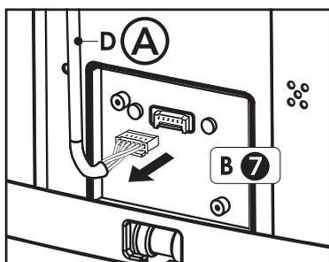
**Warning:** Do not pull on the individual cables at the plug of the control cable (D-A) as this may damage the cable!
