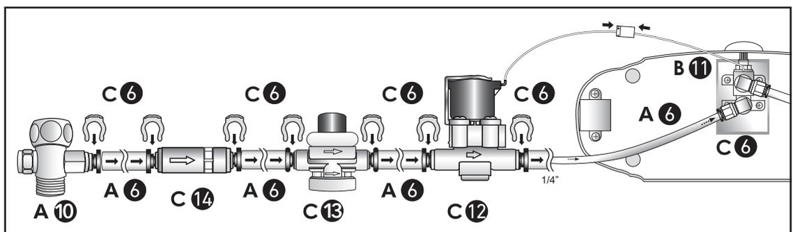
quick-release fastener opening of the water inlet (B-11) on the bottom of the ECAIA ionizer S. Finally, fix the 5 1/4" safety pins (C-6) in place. Afterwards, connect the cable of the solenoid valve (C-12) to the cable plug-in connector on the bottom of the ECAIA ionizer S.
