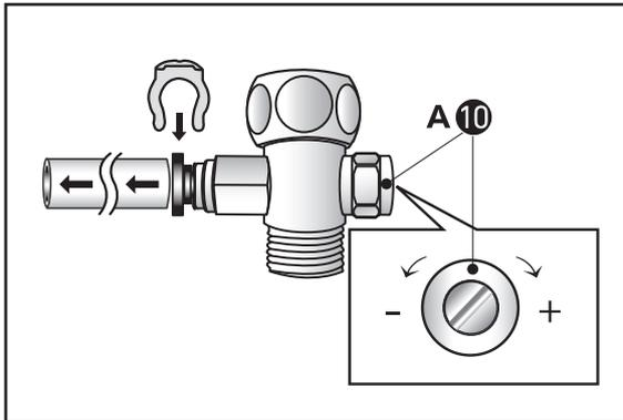
**Note:** If there is not enough water pressure, remove the water pressure reducing valve (C-13) if necessary. If the flow becomes slower after a while, the filter (A-7) and/or the water pressure reducing valve (C-13) may be dirty and may need to be cleaned or replaced.
