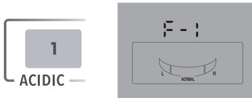
4. Press and hold on the ECAIA ionizer S the button combination "alkaline level 5" (B-24) and "PURIFY" (B-26) at the same time until the display (B-2) switches off. This saves the setting.
